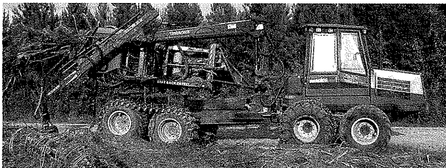
Materials are loaded onto the feed tray (end of unit on left) of the bundler unit. Feed rollers pull material into the presses (toward middle of unit).
